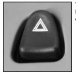
The hazard warning flasher button is located at the top of the steering column.
